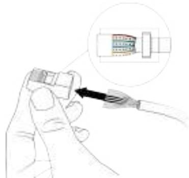
2. Connect the network cable RJ45 plug to the Ethernet socket on the communication board.
