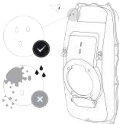
3. On the charging station, check that the feed-through seal for the display cable is correctly installed.
