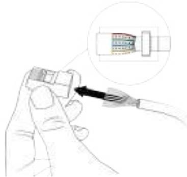
2. Connect the network cable RJ45 plug to the CT IN socket.
